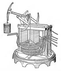
FIG. 98. Constant current transformer (G. E. Co.) showing coils, core, and counter-weight device.
